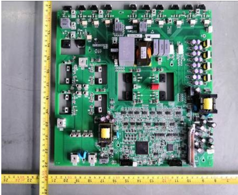
Power board view (Components side)
